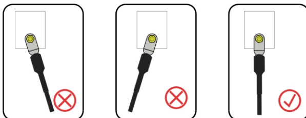
Figure 5-5 Ensuring the cables are parallel
